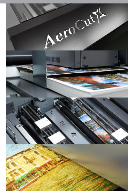
Place your printed output on the AeroCut. It automatically reads the barcode, adjusts the machine precisely and cuts! Even if page layouts change, the AeroCut adjusts on-the-fly.
