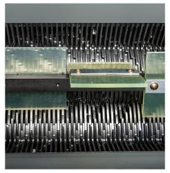
Aggressive, heavy-duty cutting cylinders are designed for high-volume shredding.
