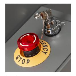
Safety features include emergency stop button and key lock to prevent unauthorized use.
