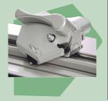
Angled cuts allows the plate to wrap around the roller leaving virtually zero gap.
