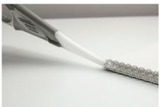
Position the nose of the Ring Wire Opener into the wire seam.
