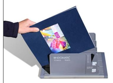
Wait for the machine to signal that the thermal binding process is complete. Remove the bound books from the heating plate. Allow the finished books to rest spine-side-down in the cooling rack for two minutes before opening.
