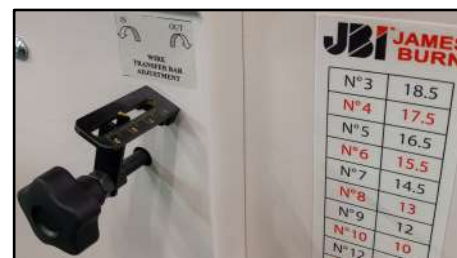
It's very easy to adjust the depth of the Wire-O® magnetic transfer bar
