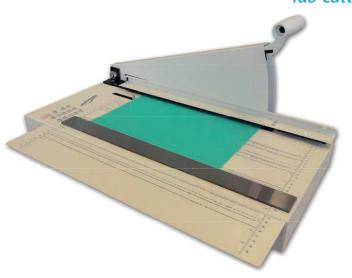
James Burn Onglématic O5 Tab Cutter is a guillotine-style index tab cutter with electric positioning and manual cutting action. This table-top unit is equipped with a choice of cutting dies that creates step tab sets.
