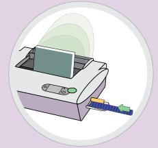
**STEP 2**: Insert binding strip into feeder.
