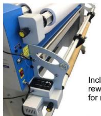
Includes motorized rear rewind with rotary slitters for roll-to-roll applications
