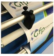
INLINE ROTARY SLITTERS trim the sides of output during lamination to save time and increase productivity.
