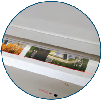
LED Laser Cut Line Shows where the blade will cut to make fine adjustments
