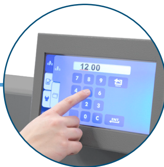
Touchscreen Control Panel Set cutting lengths, program and save up to 99 jobs, up to 30 cuts each
