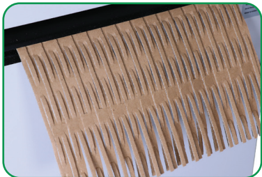
Perforation Transformation Cardboard up to .4" thick is quickly transformed into valuable net-like cushioning packing material
