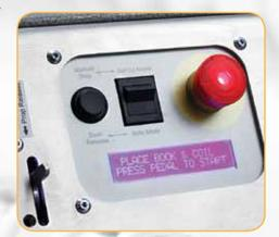
LCD Screen communicates machine status at all times.
