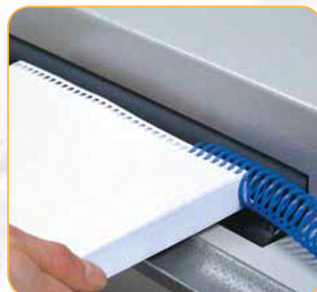
Rollers spin continuously allowing for free use of the operator's hands.
