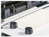
Automatic binding table clamps the media and holds the blocks in place during binding.
