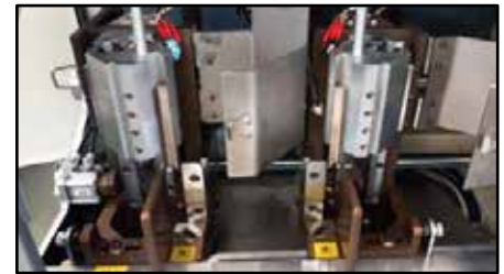
Quick and easy change of cutters with toggle clamping
