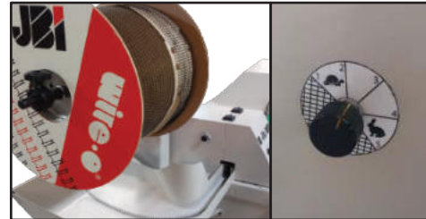
Potentiometer to adjust the trigger speed of the Wire-O® spool smoothly
