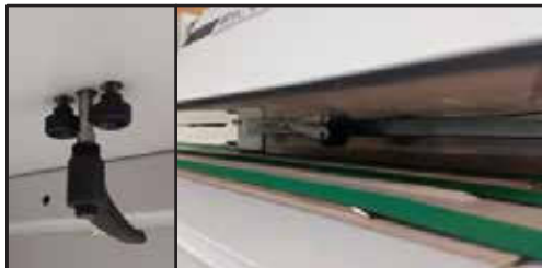
Possibility to adjust the parallelism of the Wire-O® closing area
