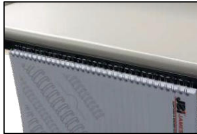
Hangers to facilitate the punching sheets insertion into Wire-O® binding
