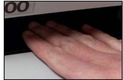
Enhanced safety with an anti-pinch protection which automatically releases the press
