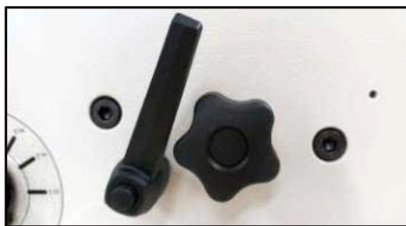
Many possible setups to adjust the parallelism of the press for a uniform closing of the Wire-O® binding
